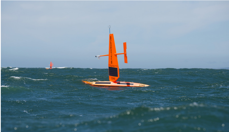
A 23-foot saildrone being tested off the coast of California can collect data on fish stocks for a fraction of the cost of a manned vessel.
